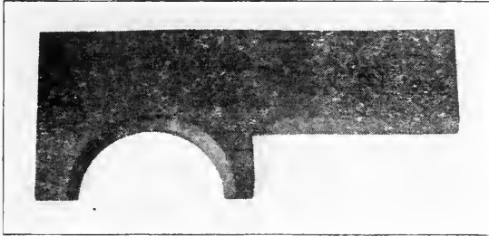
FIG. 572. TEMPLAT FOR CONVEX TURNING.
